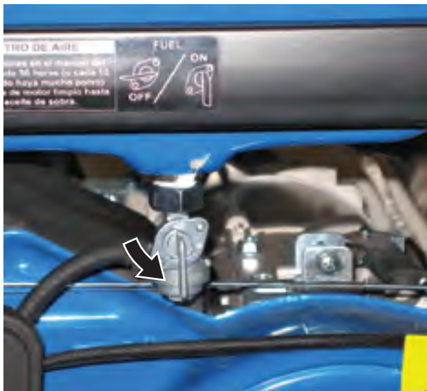
Figure 22 – Fuel Shutoff Valve in the ON Position
