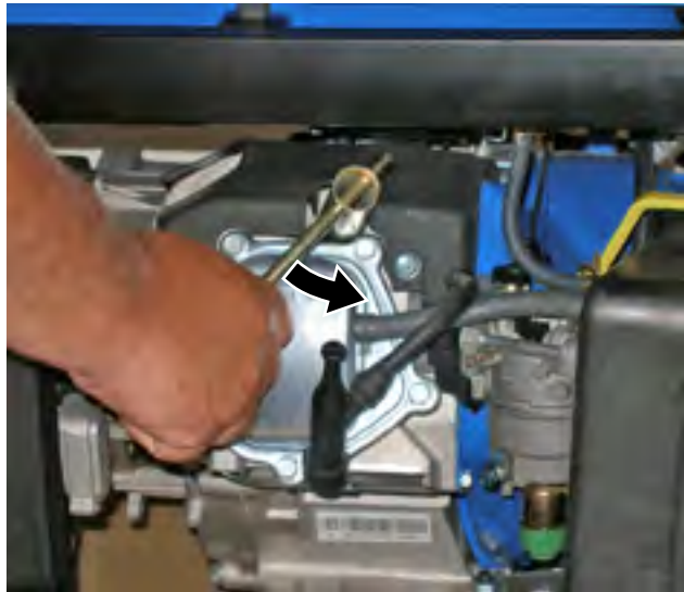
Figure 37 – Removing Spark Plug
